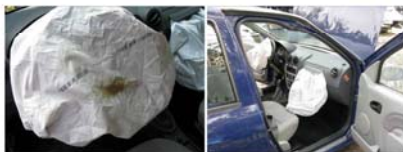
Frontal airbags with blood marks on the driver airbag
