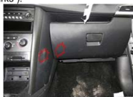
Knee marks on the lower part of compartment
