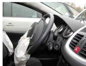
Steering wheel probably impacted by the head because of a severe impact
